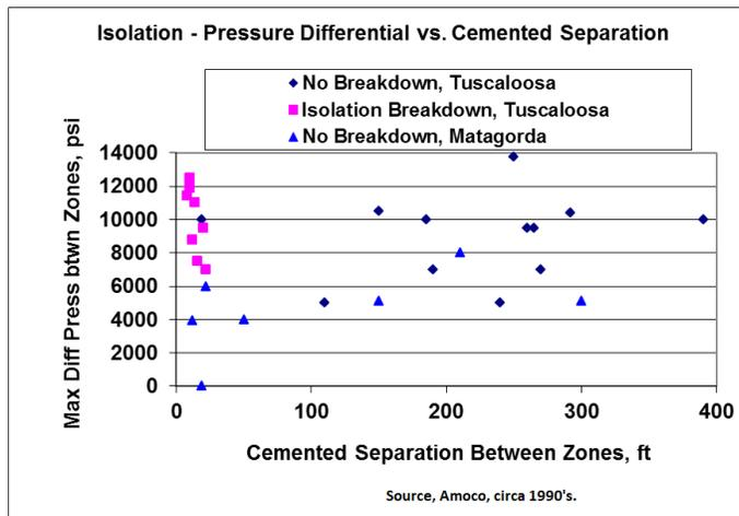
effectively isolate, shows only 25 to 50 feet of high quality cement is needed to isolate zones that have over 6,000 psi differential pressure. Common practice in the industry is to use a cement sheath that comes completely to the surface for casing that covers groundwater sources, but deeper pipe and cement pairs may use a design for a partial open annulus that allows for improved monitoring and even possible repair if a leak is detected.
